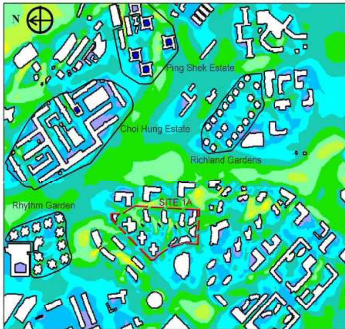
Velocity Ratio for the Proposed Scheme at pedestrian level (2m above ground)
