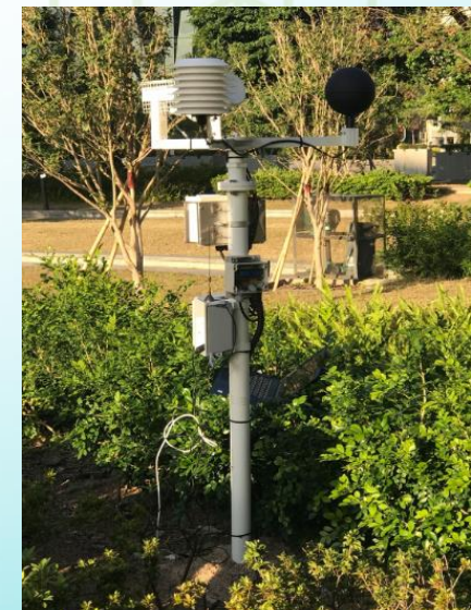
Location C – HKO's Heat Stress Monitoring System
